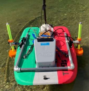
Sonar- and camera-equipped uncrewed survey vessel, L. North Santiam River, September 2024
