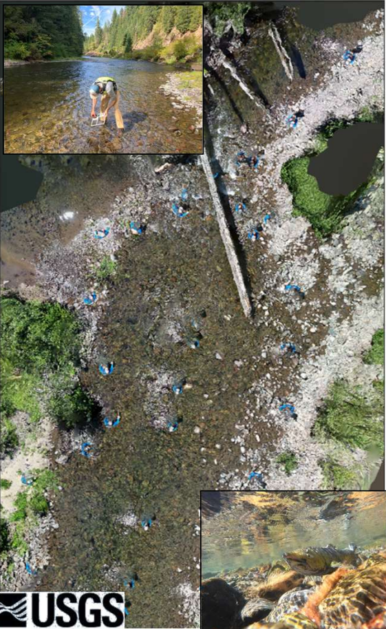
Middle Santiam River, September 2024. Orthophoto and DEM from pole-mounted camera
